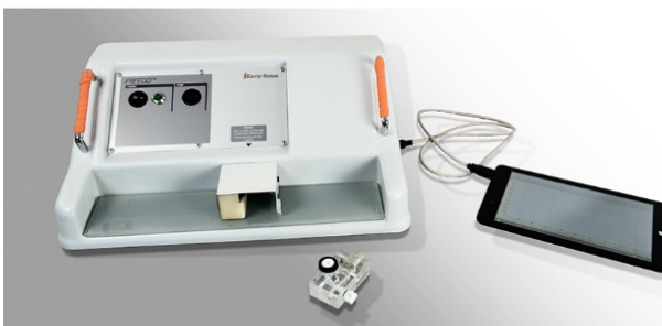
The FREEDD measuring unit with the test cell in the front.
